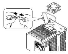
Figure 8.12 Connecting the power supply connector
