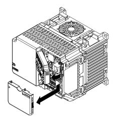
Figure 3.41 Remove the Front Cover
