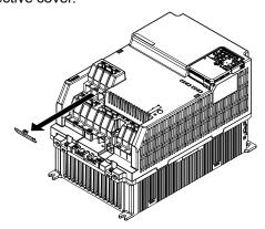
Figure 3.34 Remove IP20 Terminal Protective Cover
