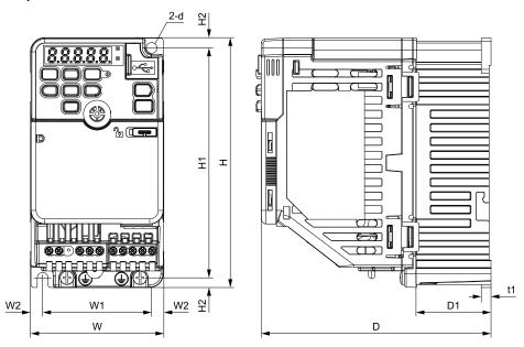
Figure 10.2 Exterior and Mounting Dimensions
