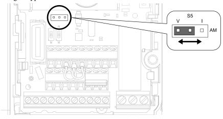
Figure 3.49 Location of Jumper Switch S5
