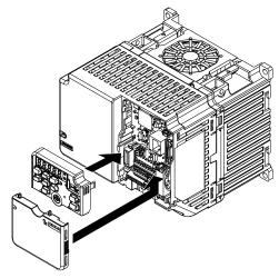
Figure 3.44 Install the Front Cover
