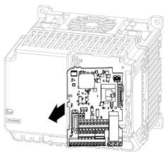
Figure 8.21 Remove the Control Circuit Board
