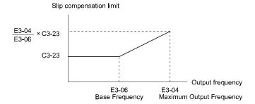
Figure 12.43 Motor 2 Slip Compensation Limit
