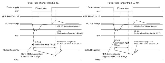
Figure 12.116 Use the KEB Ride-Thru to Cancel KEB Operation when Restoration of Power Occurs while the Control Power (Power Supply to the Control Board) is Maintained
