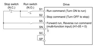
Figure 12.65 3-Wire Sequence Wiring Example
