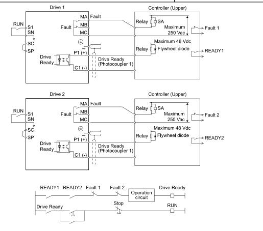
Figure 3.53 Interlock Circuit Example
