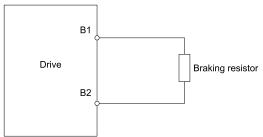
Figure 3.54 Install an ERF-Type Braking Resistor
