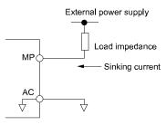
Figure 12.104 Circuit Diagram When Used as the Sinking Input
