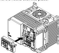
Figure 2.12 Reattach the Keypad
