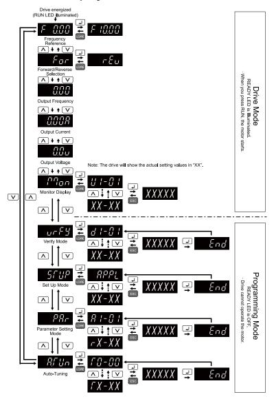
Figure 4.5 Keypad Functions and Display Levels
