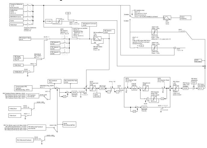
Figure 12.29 PID Control Block Diagram
