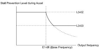
Figure 12.122 Stall Prevent Level during Accel/Limit
