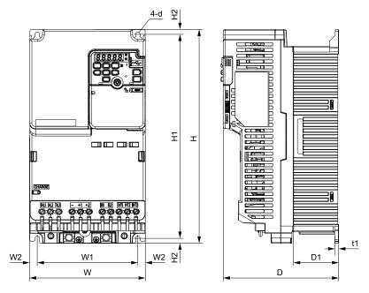
Figure 10.4 Exterior and Mounting Dimensions
