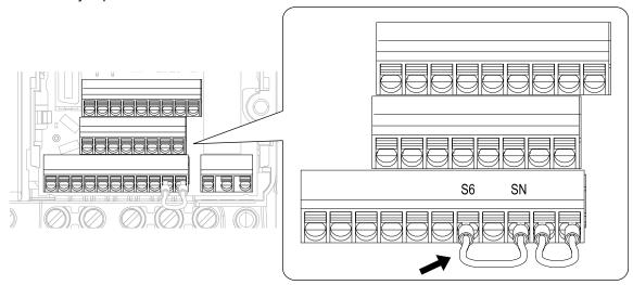
Figure 6.8 Self-Diagnostics Jumper Terminals
