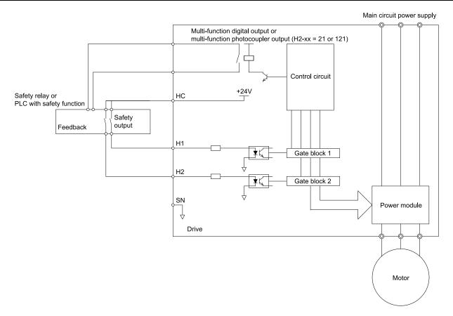
Figure 5.23 Safe Disable Function Wiring Example
