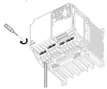
Figure 3.36 Tighten Terminal Block Screws
