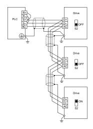
Figure 6.4 Wiring Diagram for More than One Drive
