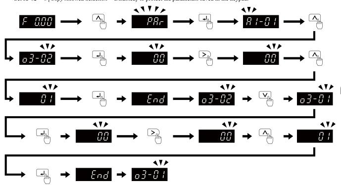
Figure 4.20 How to Save Backed-up Parameters
