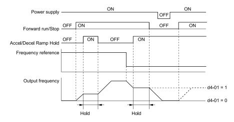
Figure 12.53 Frequency Reference Hold with Accel/Decel Hold Function
