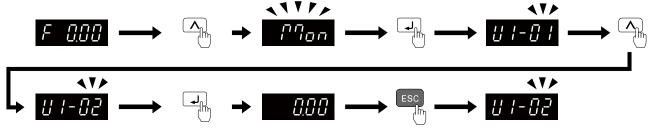
Figure 4.16 How to Monitor the Parameter Setting Values
