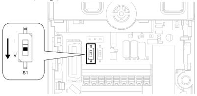
Figure 12.109 Settings for DIP Switches
