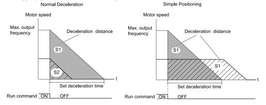
Figure 12.16 Deceleration When Set for Stop in Position
