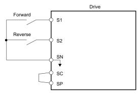
Figure 12.72 2-Wire Sequence Wiring Example
