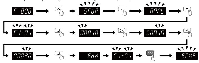
Figure 4.9 Key Operation Examples for Parameter Settings
