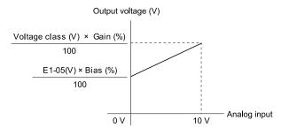
Figure 12.92 Output Voltage Bias through Analog Input
