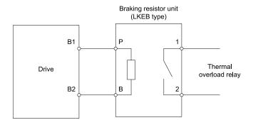
Figure 3.55 Install a Braking Resistor Unit: LKEB-Type
