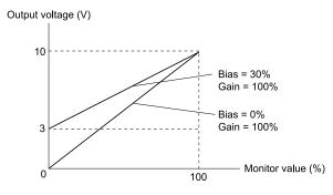
Figure 12.99 Analog Output Gain/Bias Configuration Example 2
