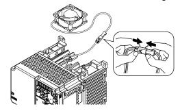
Figure 8.3 Connect the Power Supply Connector
