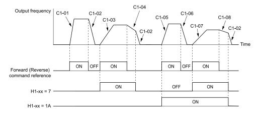
Figure 12.35 Timing Diagram of Acceleration and Deceleration Times
