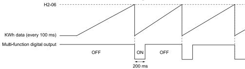
Figure 12.76 Example MFDO when Configured for Watt Hours
