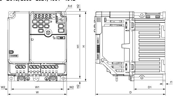
Figure 10.3 Dimension Diagram 1
