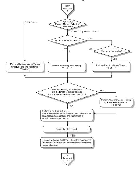
Figure 4.13 Induction Motor Auto-Tuning and Test Run Procedure
