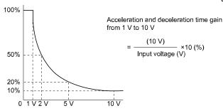
Figure 12.93 Acceleration/Deceleration Time Gain through Analog Input
