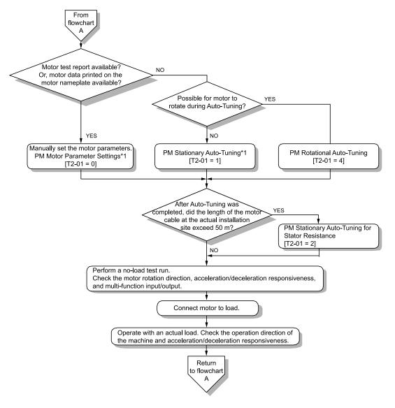
Figure 4.14 PM Motor Auto-Tuning and Test Run Procedure
