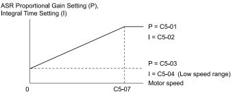
Figure 12.45 Low-speed/High-speed Gain Settings
