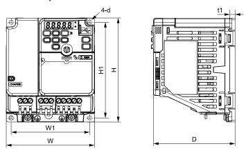
Figure 10.6 Exterior and Mounting Dimensions
