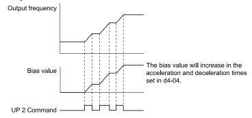
Figure 12.56 Up/Down 2 Bias when d4-03 = 0.00 Hz
