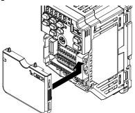
Figure 2.9 Reattach the Front Cover
