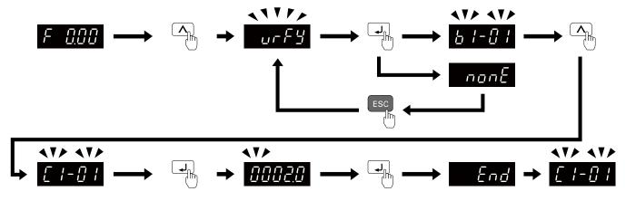
Figure 4.17 How to Examine the Changed Parameters
