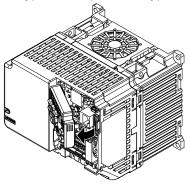
Figure 2.11 Remove the Keypad
