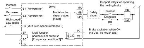
Figure 12.2 Sequence Circuit Configuration Diagram
