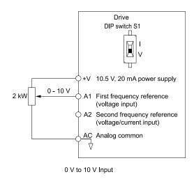
Figure 12.7 Example of Setting the Frequency Reference with a Voltage Signal to Terminal A1
