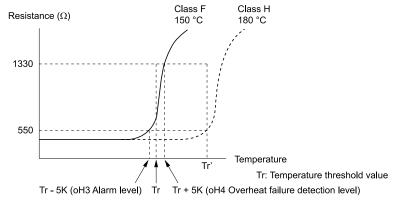
Figure 12.107 PTC Thermistor Temperature and Resistance
