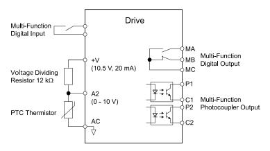
Figure 12.108 Connect Motor to PTC Thermistor Input
