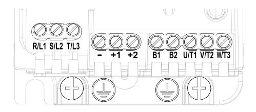
Figure 3.6 Configuration of Main Circuit Terminal Block (Three-Phase, With a Built-in EMC Filter)
