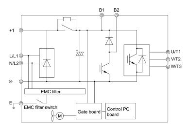
Figure 3.26 Drive Main Circuit Configuration 2
