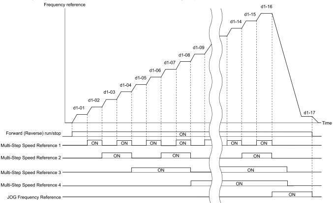
Figure 12.50 Time Chart for Multi-step Speed Reference/JOG Reference
