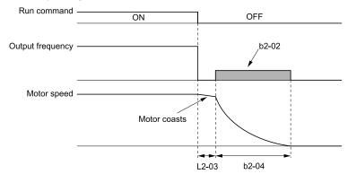
Figure 12.12 DC Injection Braking to Stop
