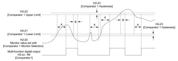
A - H2-24 [Comparator 1 On-Delay Time] B - H2-25 [Comparator 1 Off-Delay Time]
