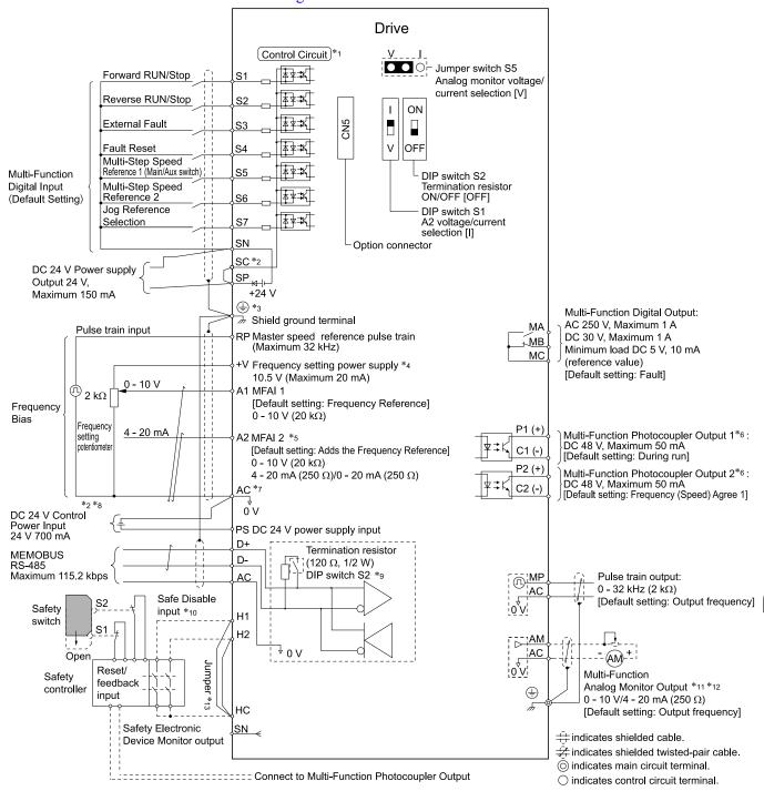
Figure 3.37 Control Circuit Connection Diagram
