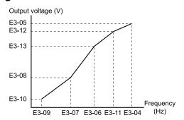
Figure 12.62 Motor 2 V/f Pattern Diagram
