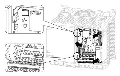
Figure 8.23 Attach the Control Circuit Board
