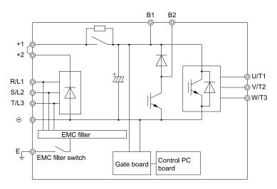
Figure 3.27 Drive Main Circuit Configuration 3
