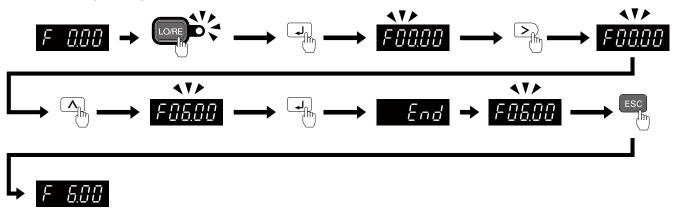
Figure 4.7 Frequency Reference Setting in Drive Mode
