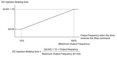
Figure 12.13 DC Injection Braking Time and Output Frequency
