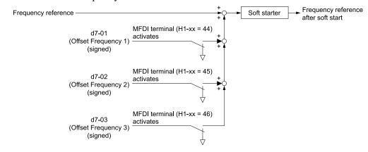
Figure 12.60 Offset Frequency Operation
