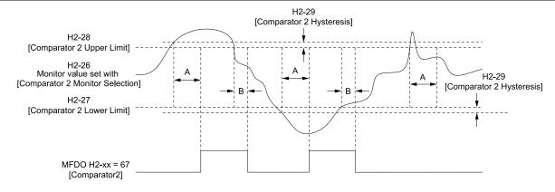
A - H2-30 [Comparator 2 On-Delay Time] B - H2-31 [Comparator 2 Off-Delay Time]
