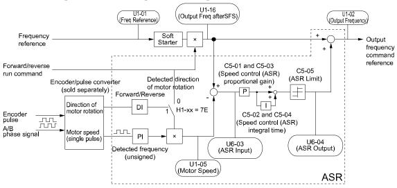
Figure 12.102 Simple Closed Loop Speed Control Block Diagram
