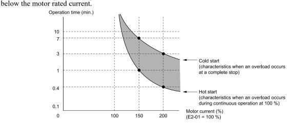
Figure 5.19 Protection Operation Time for a General-purpose Motor at Rated Output Frequency
