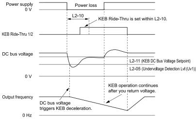
Figure 12.112 KEB Operation through KEB Ride-Thru Input
