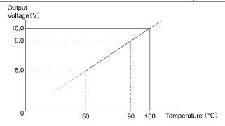
Figure 2.14 Heatsink Plate Temperature Output on MFAO
