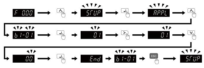
Figure 4.8 Key operation examples in Setup Mode
