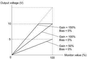
Figure 12.98 Analog Output Gain/Bias Configuration Example 1
