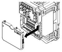
Figure 2.8 Remove the Front Cover
