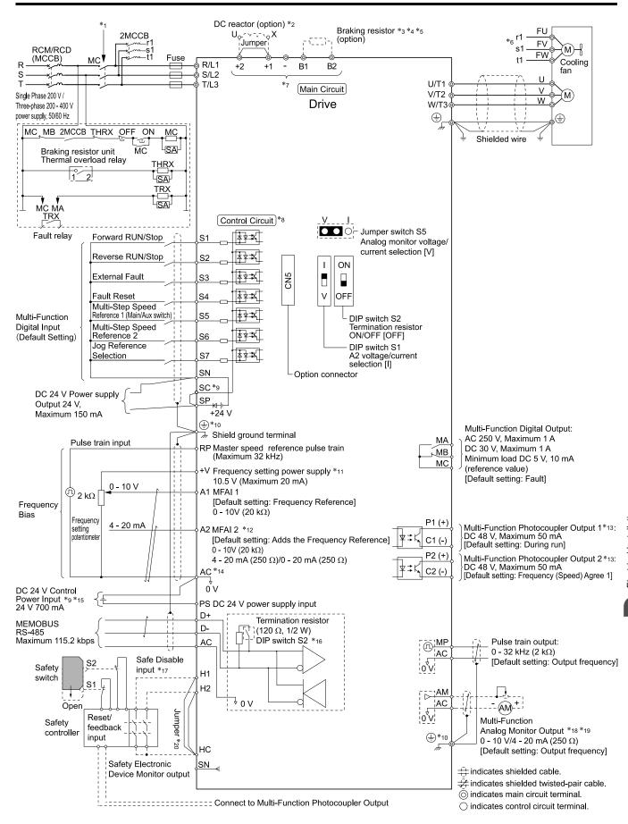
Figure 3.1 Standard Drive Connection Diagram
