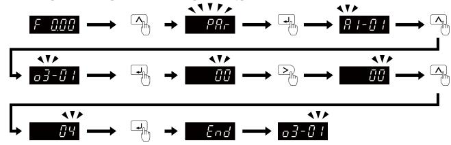
Figure 4.23 How to Erase the Backed-up Parameters
