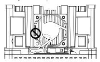
3. Put the cable and connector in the recess of the drive.
