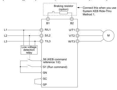
Figure 12.117 KEB Function Wiring Example
