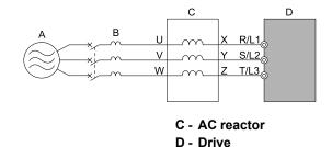
Figure 3.58 AC Reactor Connection Example
