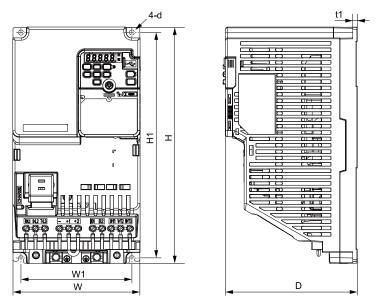
Figure 10.7 Exterior and Mounting Dimensions
