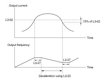
Figure 12.120 Stall Prevention During Acceleration Function in OLV/PM
