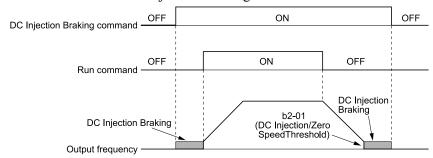
Figure 12.73 DC Injection Braking Time Chart
