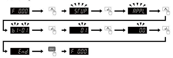
Figure 4.18 Set and View Quick Setup Parameters
