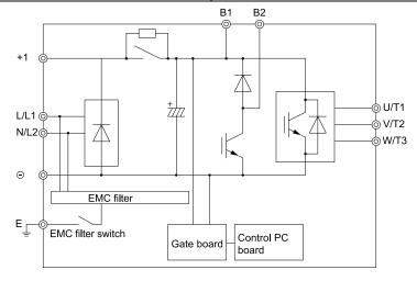
Figure 3.25 Drive Main Circuit Configuration 1
