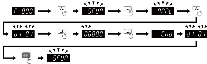
Figure 4.6 Parameters in General-Purpose Setup Mode
