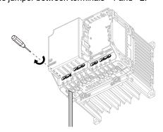
Figure 8.22 Wire the Main Circuit Terminals
