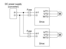
Figure 5.3 Wiring Example for DC Power Supply Input
